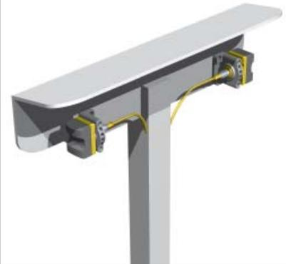
Figure 4. Install STB Buttons so that they are protected to prevent defeat or inadvertent actuation
