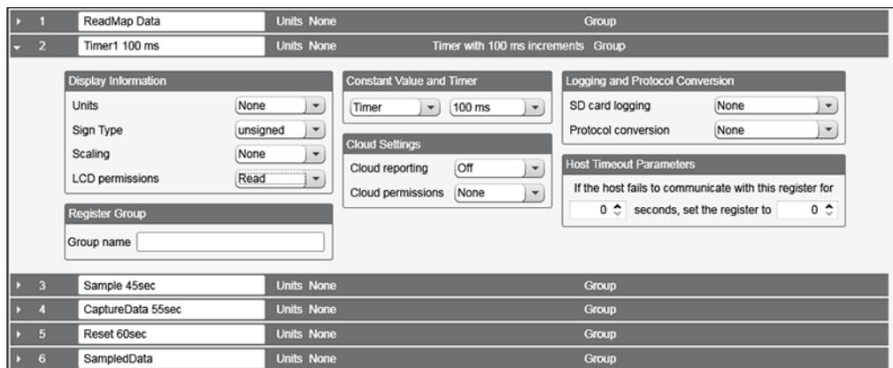
4. Name local register 3 to hold the result of Action Rule 1 (when the timer/counter reaches 45 seconds, this register value is 1).
