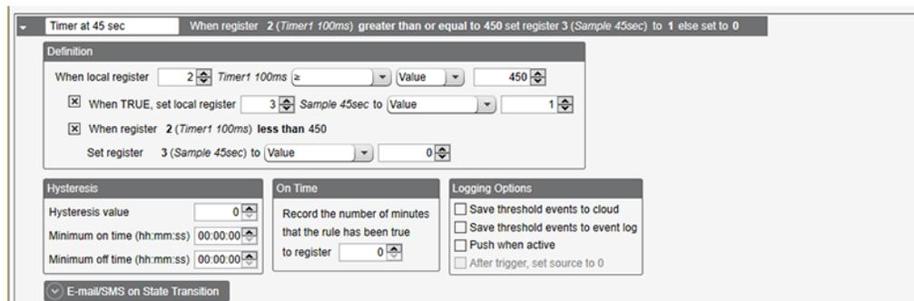
For this example, we want to check when local register 2 (the timer/counter) is greater than or equal to 45 seconds. When it does, set local register 3 to 1, otherwise, set local register 3 to zero.
