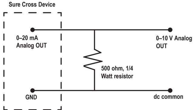
2. Connect to the same Analog OUT and GND (dc common/ground) connections in the terminal block. The instrument input tied across the 500 ohm resistor must be a high impedance input. The lower the instrument input impedance, the more offset error will be introduced.
