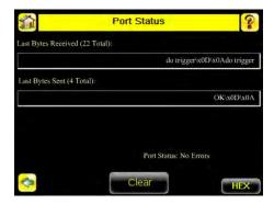
3. If the byte count does not match, re-verify that the settings on both devices match exactly. If no bytes are received, re-check the wiring.
