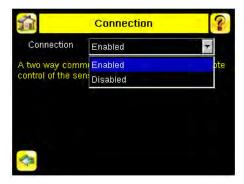
3. Configure port settings (baud rate, data bits, parity, and stop bits) on the iVu to match the settings on the control device. Go to Main Menu > System > Communications > Serial I/O.
