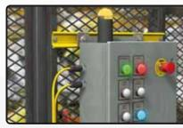
**K50L** and **K30L** dome lights (50 mm and 30 mm diameter) with a threaded base for easy installation.
