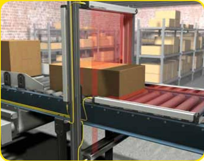
**Objective:** Measure height, length and width of boxes for storage and collect profile information for shipping.
