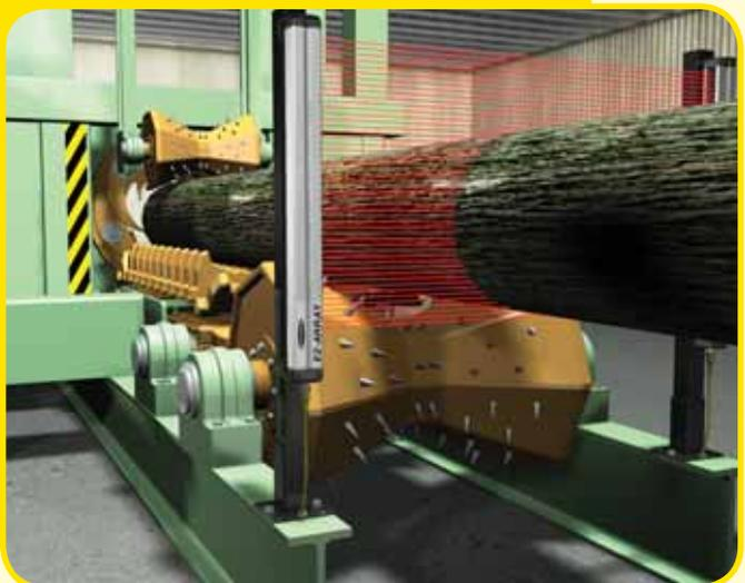
**Objective:** Determine the diameter of a log before it has entered a station used for bark removal.
