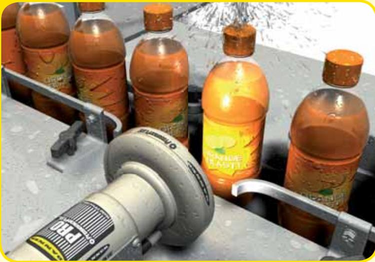
**Objective:** To confirm that each soda bottle in a wet environment has a label in the correct position.
