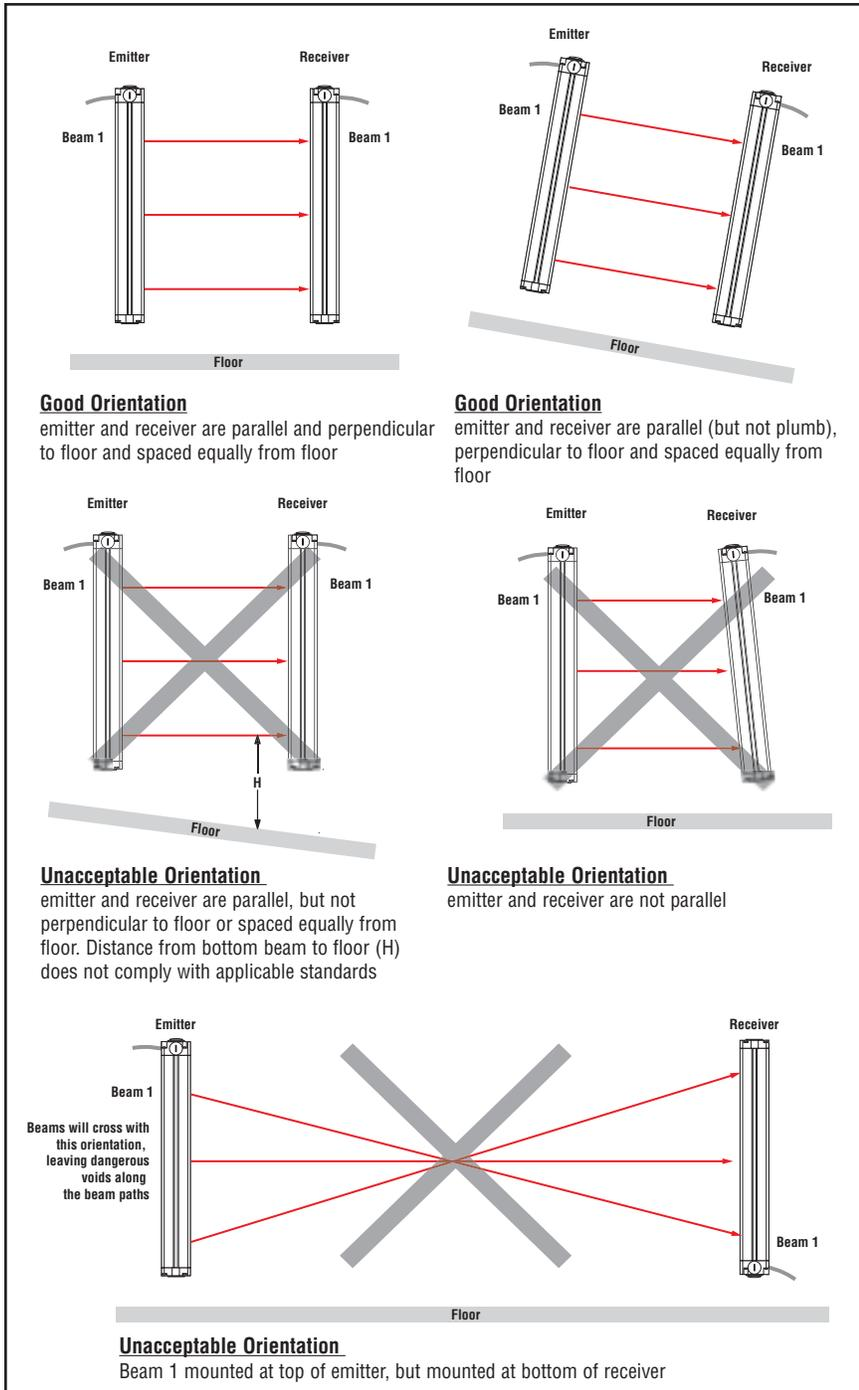
Figure 3-5. Emitter/receiver orientation
