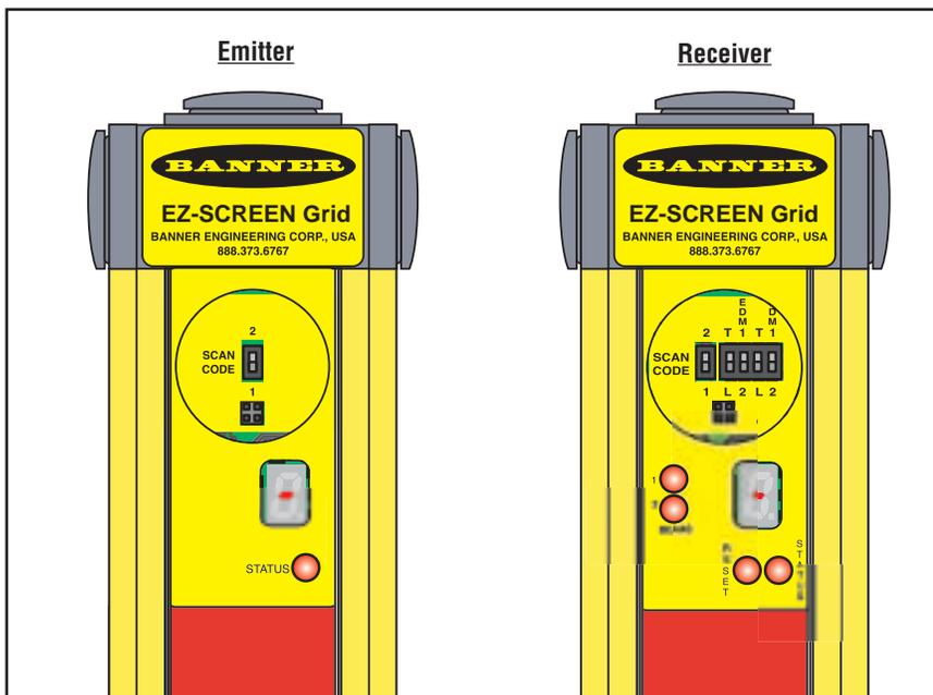
Figure 4-1. EZ-SCREEN Grid configuration switches
