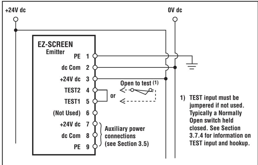
1) TEST input must be jumpered if not used. Typically a Normally Open switch held closed. See Section 3.7.4 for information on TEST input and hookup.
