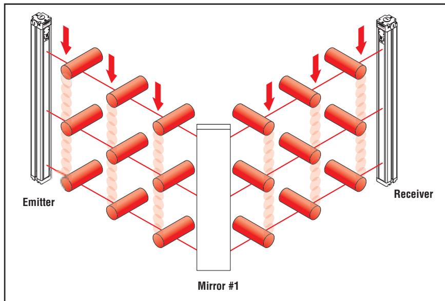
Figure 6-2. EZ-SCREEN Grid trip test with corner mirrors
