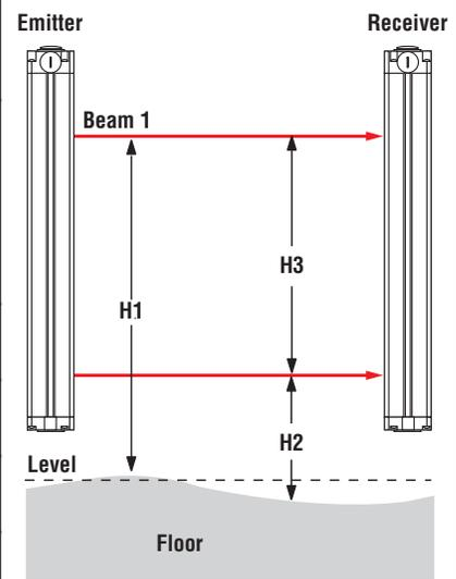
Figure 3-10. Verify required height between the top and bottom beams and the floor, throughout the length of the beam path, per applicable standards.
