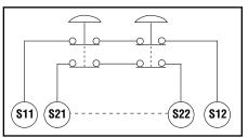
Figure 2. Series connection of multiple E-Stop switches. Jumper between \$21 and \$22, if 1-channel E-stop is selected.
