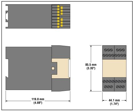
Figure 8. E-Stop Safety Modules ES-TN-1H.. enclosure dimensions
