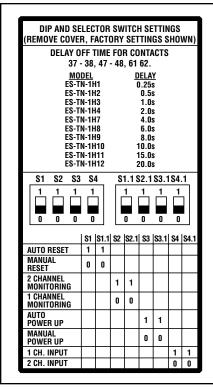
Figure 6. Module DIP switches and selectors, set to factory settings
