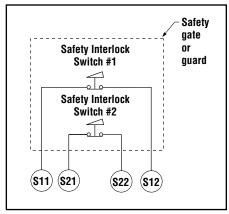
Figure 4. Hookup using contacts from two safety switches
