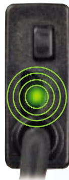
Green Flashes five times to indicate maximum gain
