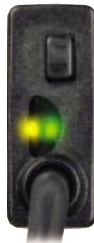
Green Steady: Power on Amber Steady: Light sensed
