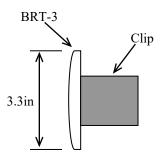
As the red laser beam strikes the clipon target, the BRT-3 reflector will "glow" a bright red. When the beam strikes the mounting screw the "glow" will dim slightly. At this point, if the LAT-1 and the Clip-on target are mounted at the same point on a plumb emitter and receiver, the two points should be approximately the same distance above a level floor.
