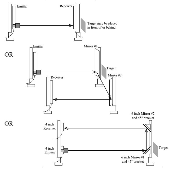
10) Rotate or otherwise adjust the physical positioning of the emitter so as to place the red dot at the same approximate position on the receiver (or mirror) (distance from the end of the unit) as the red line on the LAT-1 label is positioned on the emitter. (See above). When aligning multiple mirrors, the important key is to "work around" from one mirror to the next to place the red dot on the opposite sensor.
