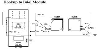
The SM53E/SM53R sensor pair has an analog output which serves as the input to a B4-6 ac-coupled amplifier. *Note that the white wires from both emitter and receiver tie together at the amplifier input.* This connects together the AGC circuit which regulates the emitter output for constant received light signal strength. The model MRB chassis (shown) operates from 120V ac and provides +15V dc to the sensors and amplifier module.
