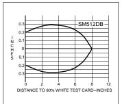
Model **SM512DB** is a **short-range proximity mode sensor** for applications requiring fast response time, such as leading-edge detection in carton-flap gluing installations or presence sensing for triggering high-speed ink-jet type imprinters.
