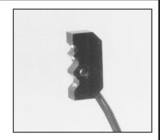
**Model SP100AF** is an adjustable-field convergent mode sensor that detects objects directly by reflection of light from the object's surface. Objects in the background are ignored, regardless of their surface reflectivity.
