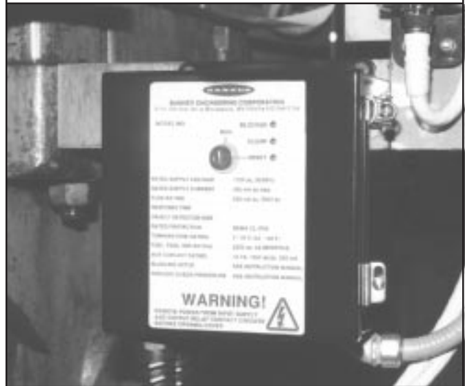
Figure 4. A MACHINE-GUARD System Control Box. The system described in this manual uses model MGCA-5A or MGCB-5A.
