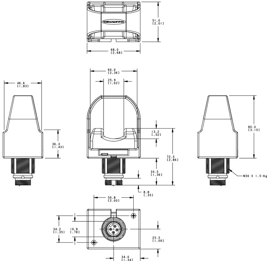
Figure 2. OTB with M12 Quick-Disconnect
