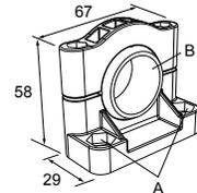
Hole center spacing: A =  $\varnothing$  50.8
