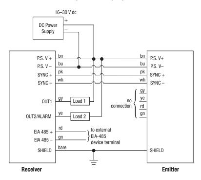
Figure 2. PNP Wiring Diagram
