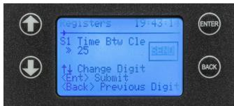
1. Using the up and down arrow buttons, select the first digit and press **ENTER** to set the first digit.
