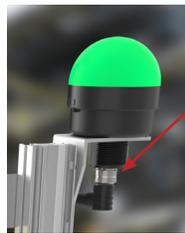
2. Connect the power supply to the Indicator Light, aligning the keys in the connector. Hand tighten.
