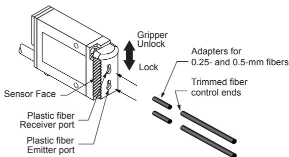
Figure 1. MINI-BEAM with fiber grippers
