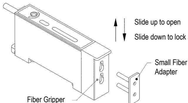
1. Cut the fiber ends according to the instructions included with the fibers.
