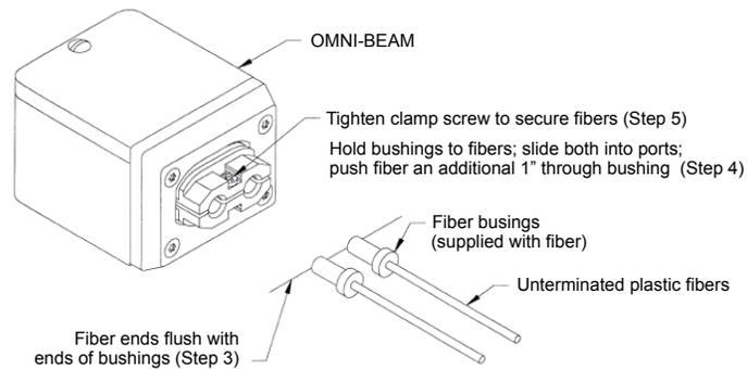
1. Prepare the sensor ends of the fibers (see [Cut the Plastic Fiber](#) on p. 3).
