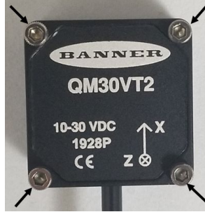
QM30VT2 screwed onto the BWA-QM30-FTAL bracket
