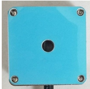
BWA-QM30-FTAL with the blue thermal tape liner facing up
