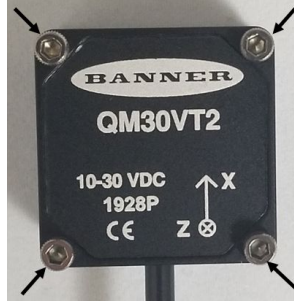
QM30VT2 mounted to the BWA-QM30-FMSS bracket
