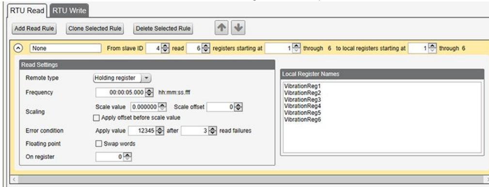
1. From the **Register Mapping > RTU > RTU Read** screen, click **Add Read Rule**.
