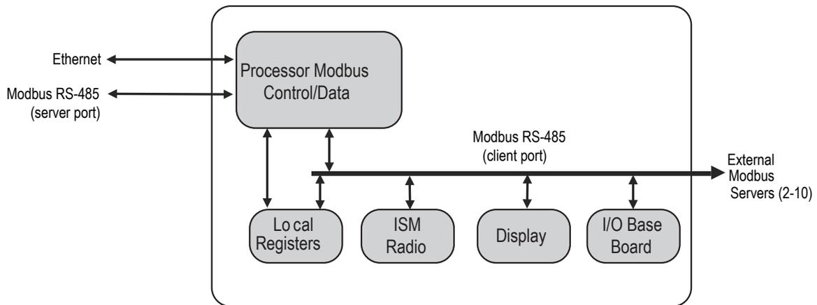
The DXM has dual Modbus roles: a Modbus server device and a Modbus client device. These run as separate processes.
