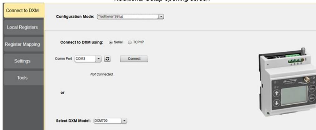
Connect via USB or Ethernet. If connecting via Ethernet, set network parameters through the DXM LCD menu in the **System Cfg > Ethernet** menu. Network parameters can also be set within the configuration software. Setting parameters on the LCD menu overrides the parameters stored in the configuration file. To use the network parameters in the configuration file, reset the network parameters on the DXM LCD menu.
