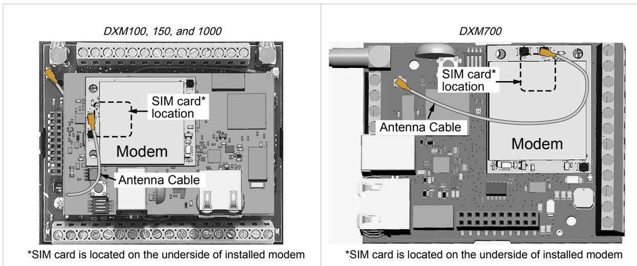
\*SIM card is located on the underside of installed modem
