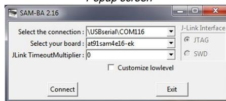
The SAM-BA program attempts to automatically detect the COM port and the correct device.
