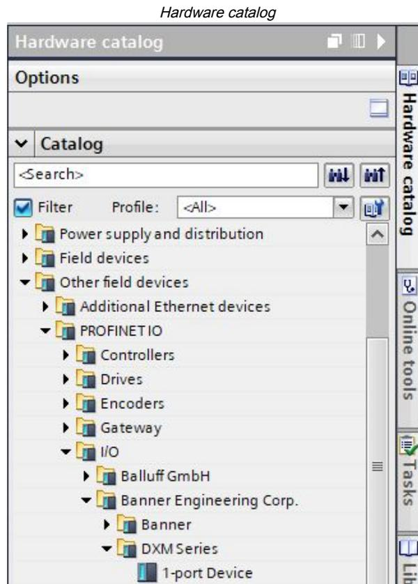
The system installs the DXM GSD file and places it in the **Hardware catalog**. In the example, the DXM GSD file is located under **Other field devices** > **PROFINET IO** > **Banner Engineering Corp.** > **Banner**.
