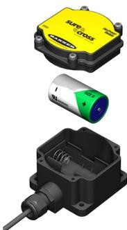
For outside or high humidity environments, dielectric grease may be applied to the battery terminals to prevent moisture and corrosion buildup.
