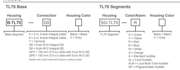
Select the 5-pin base for tower light configurations of up to 4 modules. Select the 8-pin base for tower light configurations of up to 6 modules.
