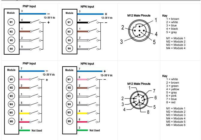
NOTE: Models SG-TL70-ALM and SG-TL70-ALMC are not compatible with NPN input wiring.
