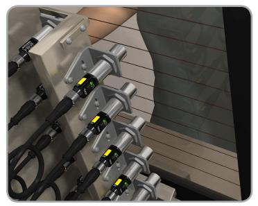
T-GAGE sensors are installed in rear window test equipment. The solution helps the supplier verify that each defrost wire heats to specification prior to shipping the product to the automotive assembler.
