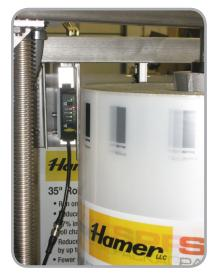
The R58 Expert accurately senses registration marks on a web of ice packaging as it passes through a high-speed, automated bagging machine.
