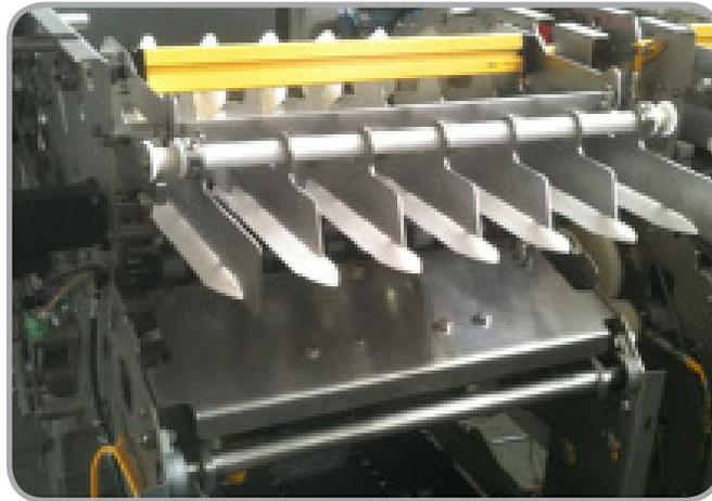
*Q20 arrays are installed on an egg sorting and packaging machine; one detects eggs as they are dropped into sorting chutes, and the second sees that the eggs are properly placed in their cartons.*
