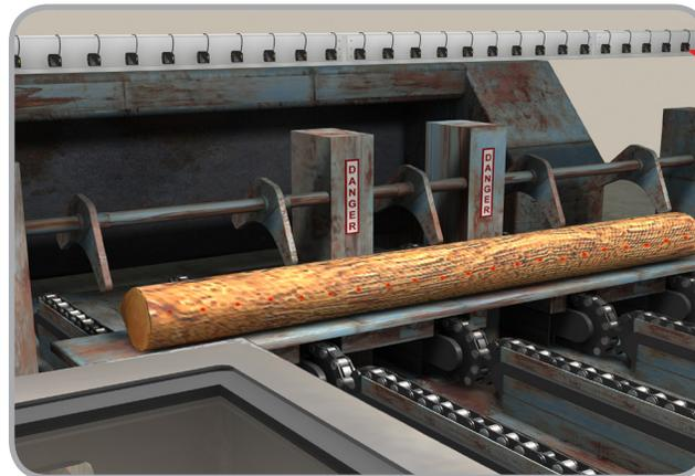
The automated lumber carriage system picks a log, clamps it and brings it to the saw for milling. An array of LT3s above the carriage are used to detect and measure various points along the log.
