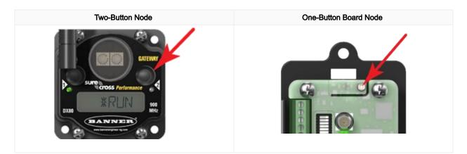
The Node enters binding mode and locates the Gateway in binding mode.
