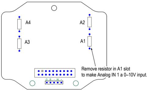
Step 1. Cut out the resistor installed in the A1 (analog 1) slot. (Your wiring board may differ slightly from the board shown. Use the board's labels to confirm you have selected the correct resistor to cut.)
