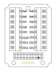
Figure 3. P7C model wiring board
