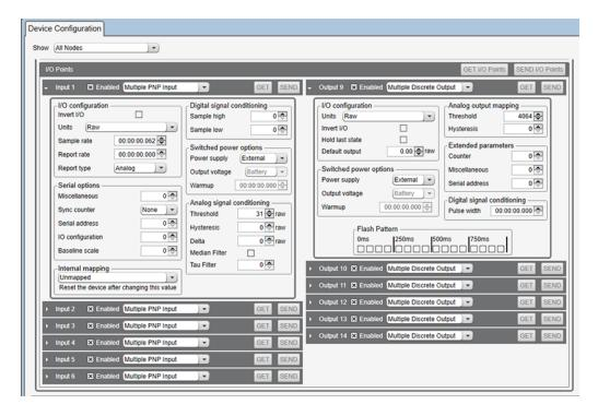
5. Click Send or Send I/O Points to upload the settings to the wireless network.
