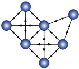
**Pros**—Information has multiple communication paths to the gateway; the gateway can be positioned anywhere in the network; and chattering nodes are removed from the network.
