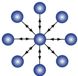
**Pros**—The gateway maintains a communications connection with each node on a separate communications path; if communication between one node and the gateway fails, the rest of the network is unaffected; and chattering nodes are removed from the network.
