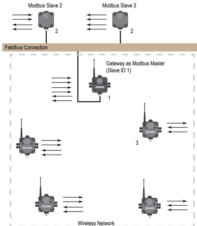
As shown, the DX80 Gateway is a slave device within the Modbus network but remains the master device of the wireless network. In this way, the DX80 Gateway behaves as a true networking gateway by bridging communications between the wireless network and the Modbus RTU network.
