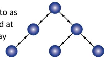
**Mesh** - To improve the reliability, network designers developed an architecture called a mesh. In a true mesh network, each node has limited routing capabilities and maintains a network connection with at least two other nodes. That way, if one link breaks, information has an alternative path to the gateway. The gateway in this case could be any one node in the network.
