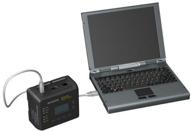
Figure 3. USB connections: PC to Safety Controller USB port connection
