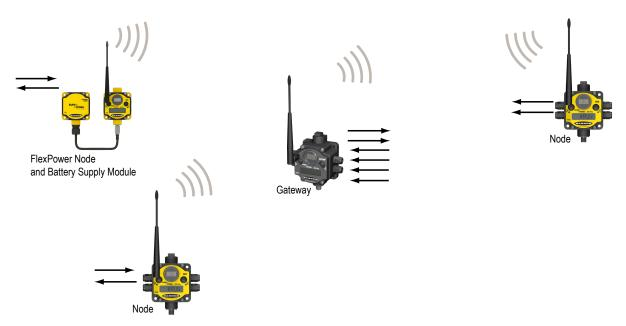
The SureCross DX80 network is a deterministic system—the network identifies when the radio signal is lost and drives relevant outputs to user-defined conditions. Once the radio signal is reacquired, the network returns to normal operation.
