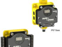
The SureCross™ wireless system is a radio frequency network with integrated I/O that can operate in most environments while eliminating the need for wiring runs. Systems are built around a Gateway, which acts as the wireless network master device, and one or more Nodes. A remote I/O device with a Modbus interface is used to expand the I/O of the Gateway device or the Modbus host.
