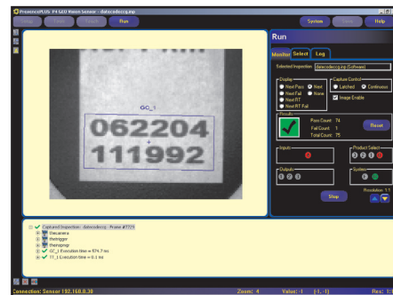
Incorrect part number "062204"
