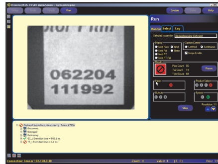
✗ Incorrect part number "062204" fails
