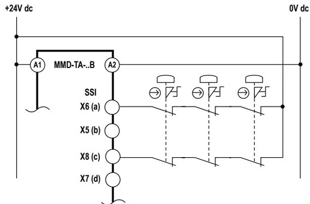
Figure 24. SSI Category 3 interfacing: positive-opening E-stop switch(es)
