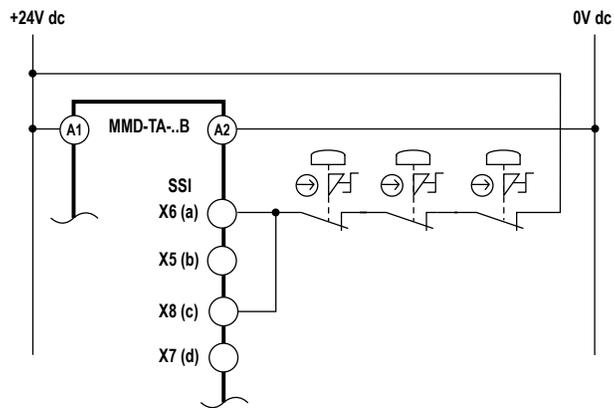
Figure 23. SSI Category 2 interfacing: positive-opening E-stop switch(es)
