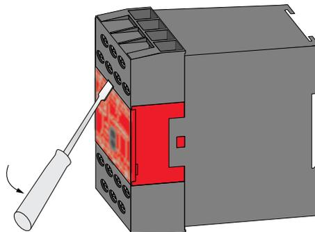
Figure 7. Removal of Terminal Blocks
