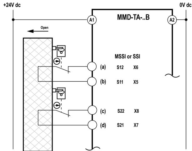
Figure 28. SSI Category 4 interfacing: positive-opening interlocking switch(es)
