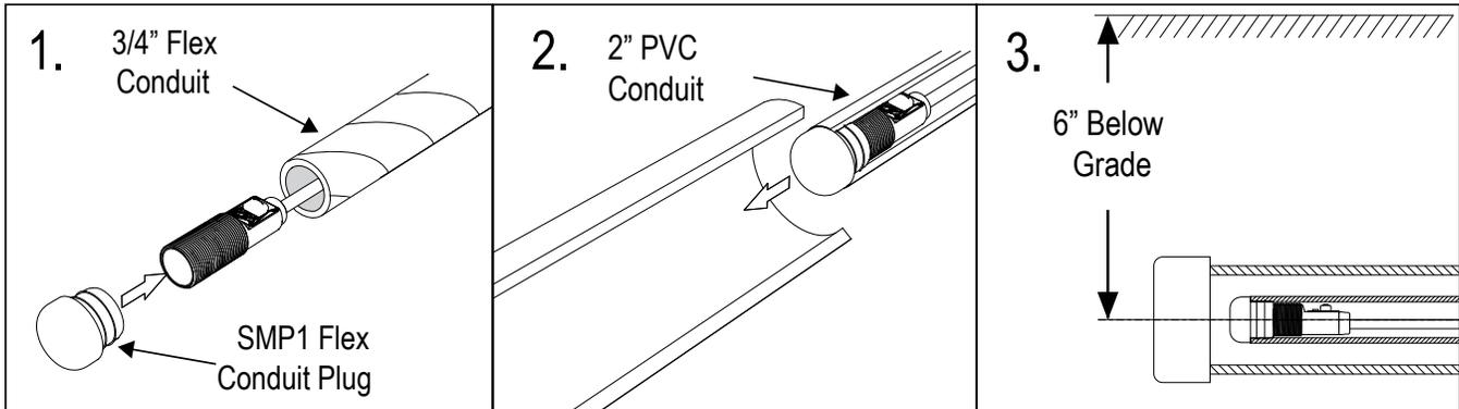
Figure 5. Below-grade installation
