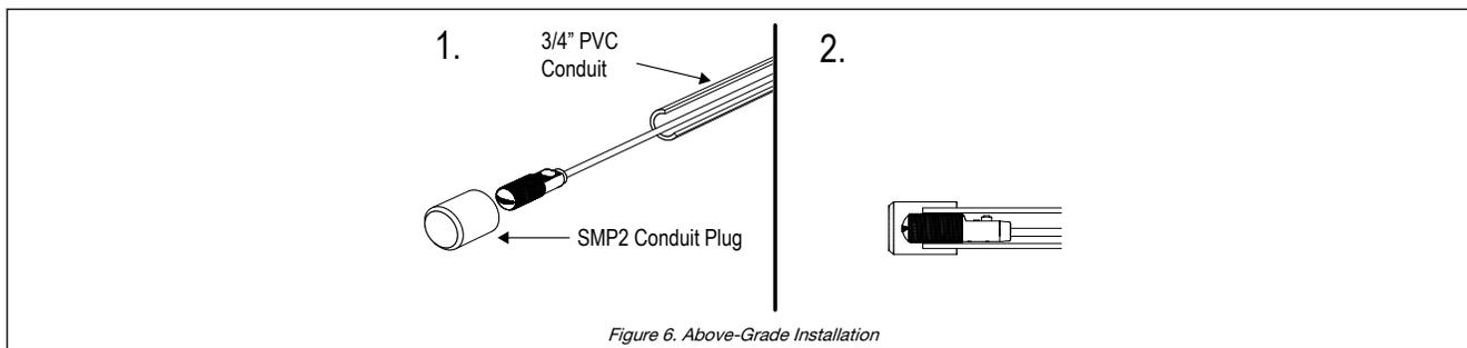
1. Mount the PVC electrical conduit from the sensing point to the control panel. Plastic conduit should be used for at least the first 6.1 m (20') from the sensing point; metal or flexible conduit may be used the remainder of the distance.
