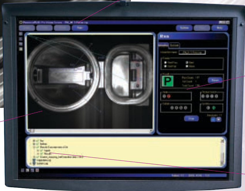
Configuration Window allows the user to select options and run inspections.
