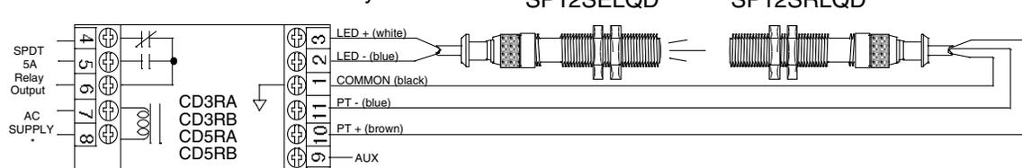
\*105 to 130V ac or 210 to 250V ac, 50/60Hz, depending on model. To power the MAXI-AMP™ module from a dc supply, connect +12 to 28V dc at 70mA to terminal #3 and dc common to terminal #1. Make no connection to terminal #7 or #8.
