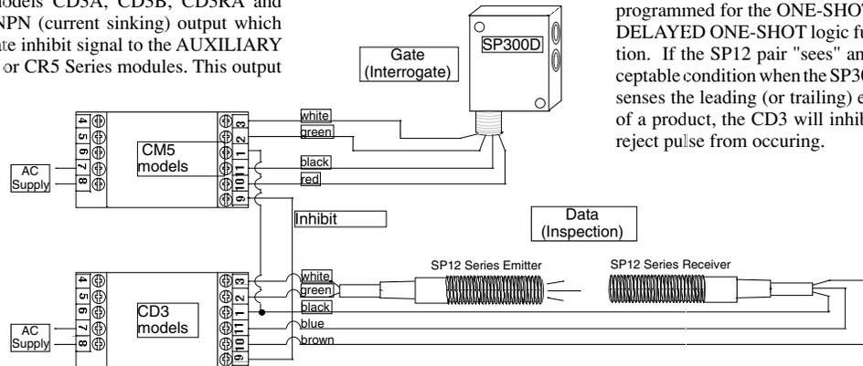
Typically, the CM5 module would be programmed for the ONE-SHOT or DELAYED ONE-SHOT logic function. If the SP12 pair "sees" an acceptable condition when the SP300D senses the leading (or trailing) edge of a product, the CD3 will inhibit a reject pulse from occurring.
