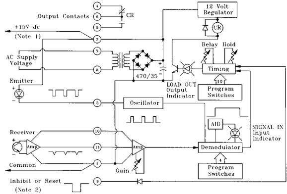
**NOTE #1:** power is available at pins #3 (+) and #1 (-) for an external 10 to 30V dc device (see hookup example, page 3). Current available is 40 mA at 120V ac (240V ac) line level; 30mA at 105V ac (210V ac) line level. Alternately, the module may be powered by 12 to 28V dc at pins #3 (+) and #1 (-). Do not connect ac voltage when using external dc power.
