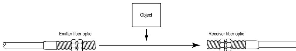
1. To align two individual fiber optic assemblies for opposed mode sensing, begin with one sensing tip mounted firmly in place.
