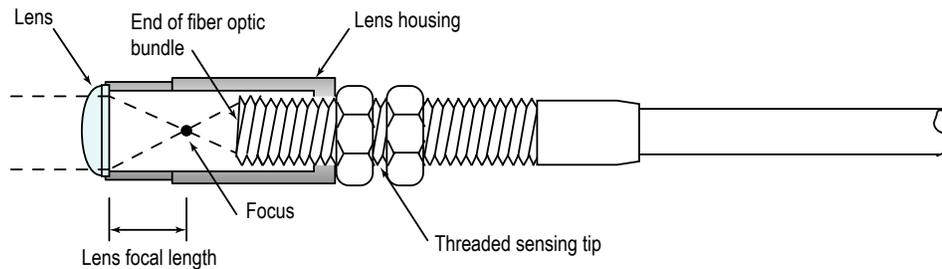
1. Illuminate the bundle at the threaded end of the fiber optic assembly by holding the opposite end toward a visible light source.
