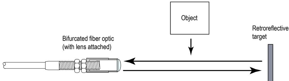
Sensor block models SBF1, SBF1MHS, or SBFV1 are used with a BT13S fiber and an L9 or L16F lens assembly for retroreflective sensing. Unlike most two-lens retroreflective sensing designs, a bifurcated fiber optic/lens combination has no minimum sensing distance. As a result, this combination is an excellent choice for retroreflective sensing across small parts conveyors or for high-speed retroreflective code reading applications.
