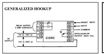
SMI912 Series sensors are certified intrinsically safe ONLY when used with certified energy-limiting intrinsically-safe barriers. Banner does not itself manufacture intrinsically-safe barriers. Barriers may, however, be purchased from Banner as part of a kit which includes one CI3RC current trip point module, one module socket, one 70mm length of DIN rail (for mounting of socket), one DIN rail barrier mount, and one (in kit model CIBK-1) or two (in kit model CIBK-2) certified barriers.
