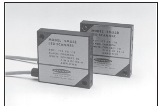
Figure A.55. Models SM53E and SM53R, a modulated opposed mode emitter and receiver pair, are useable with ac-coupled amplifiers.
