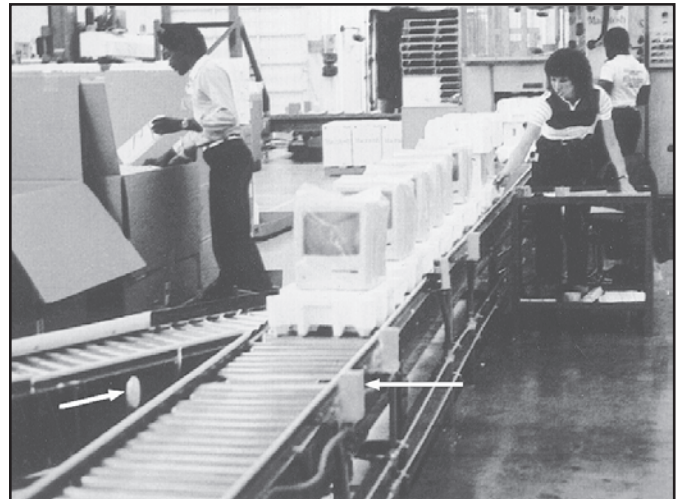
Figure B.3. The retroreflective mode is popular for many conveyor applications.
