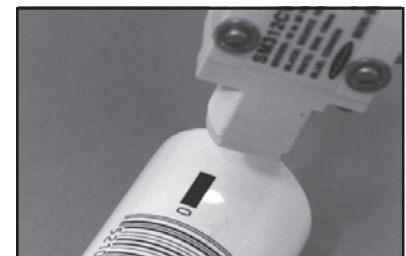
Figure B.40. Visible convergent beam sensors are a good solution to many color mark sensing applications.
