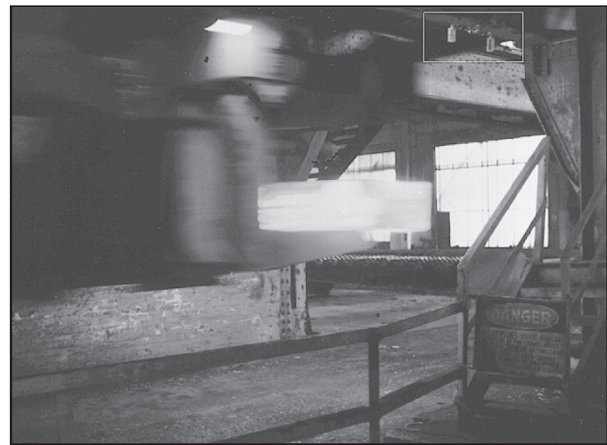
Figure B.35. Two MULTI-BEAM Ambient Light Receivers (at upper right) detect passage of red-hot steel in a steel mill.
